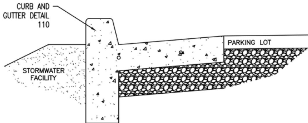
Curb and gutter detail showing deep curb used to improve stabilization and integrity of the adjacent parking lot. Engineering detail from the Low Impact Development website ([centralcoastlidi.org](http://centralcoastlidi.org)).
