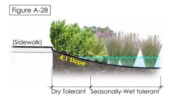
Typical Side Slope and Flat-Bottom Planting Condition
