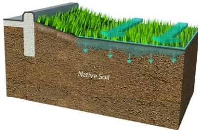
Figure 3. A bioswale facility removes pollutants primarily through filtration and settling as stormwater moves over the surface of the vegetated area. Infiltration into the native soil is negligible if a liner is used.
