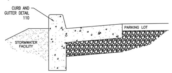
Curb and gutter detail showing deep curb used to improve stabilization and integrity of the adjacent parking lot. Engineering detail from the Low Impact Development website (centralcoastlidi.org).
