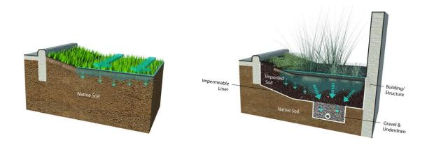
Figure 3. A bioswale facility removes pollutants primarily through filtration and settling as stormwater moves over the surface of the vegetated area. Infiltration into the native soil is negligible if a liner is used.
