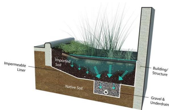
Figure 4. A bio-filtration facility infiltrates stormwater through a special soil media designed to remove pollutants. Treated stormwater is then routed through an underdrain to exit the system. Infiltration into the native soil is negligible or non-existent if a liner is used to protect foundations.
