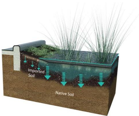
Figure 5. A rain garden or bioretention facility without an underdrain infiltrates the entire design storm to provide both stormwater quality treatment and volume reduction. Special soil media for treatment is not required.
