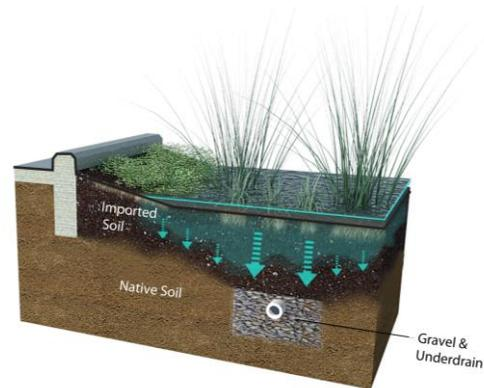
Figure 6. A bioretention facility with an underdrain is used when the native underlying soils do not adequately infiltrate, and additional subsurface storage is needed to manage the design storm. The underdrain also reduces excessive ponding duration that can occur due to the poor infiltration. Specialized soil media is used to ensure that any stormwater exiting via the underdrain has been adequately treated.
