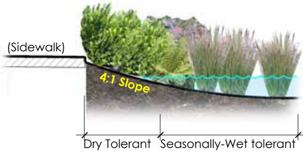
Typical Side Slope and Flat-Bottom Planting Condition
